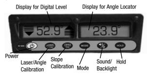
The instrument has six operating keys with their functions below:
