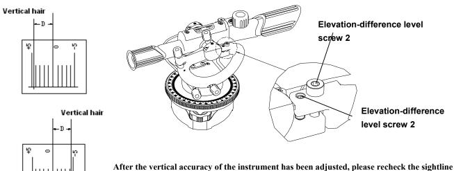
levelness of the instrument with the same method as above. If the sightline levelness is beyond tolerance, it is necessary to make readjustment.
